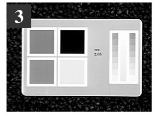
The card should be as shown, with Yellow-Magenta-Cyan-Black panels, a Cyan background and Yellow-Magenta-Cyan graduated scales. This card can only be printed by a printer in isolation, when using UR1 Dye Film
